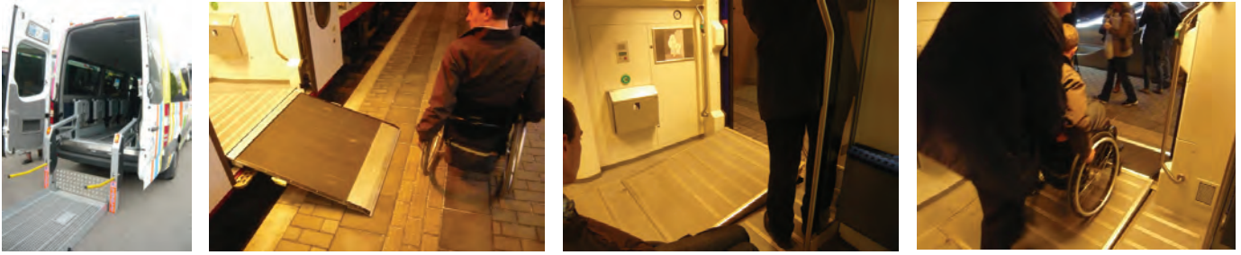
Photos: Technologies to improve mobility of people in wheelchairs: truck and bus treadmill to bridge the gap between platform and train (© Lorenzo Lucchini, 2013)
